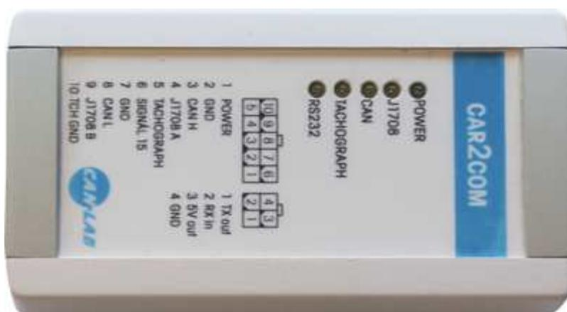
When BT module is not used, however RS232 is connected the second connector is attached. Then 4-pin connector MOLEX is attached.
